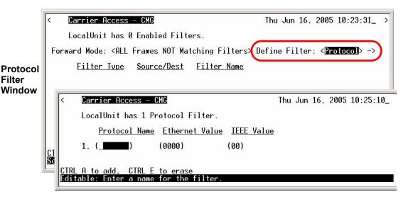
Use this screen to define filters that are based on specific protocols being used by LAN devices. These filters, when enabled, provide security by restricting LAN/WAN access based on a specific protocol.
